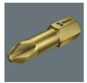
TH-Bits are hard bits with a torsion zone. Torsion bits absorb the damaging peak torque loads in the torsion zone. This prevents premature wear and enhances the service life of the bits.
